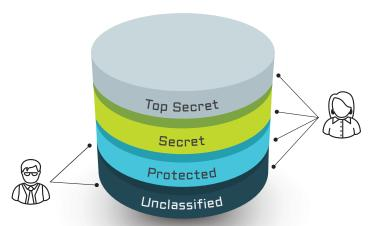
An MLS capability (system, platform, or environment) allows information at different classifications to be stored and accessed within a single security domain, while enforcing different access policies and compartments dynamically depending on context, with the assurance that the separation is effective.
